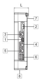
1 Serial port 2 Power supply 3 Ethernet port 0 (10/100/1000 Mb)
