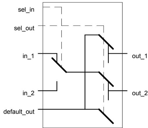
Short description: Double independently operated real switch with two inputs
