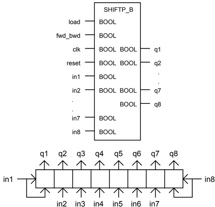
**Short description:** Bidirectional boolean shift register with 8 parallel inputs and outputs
