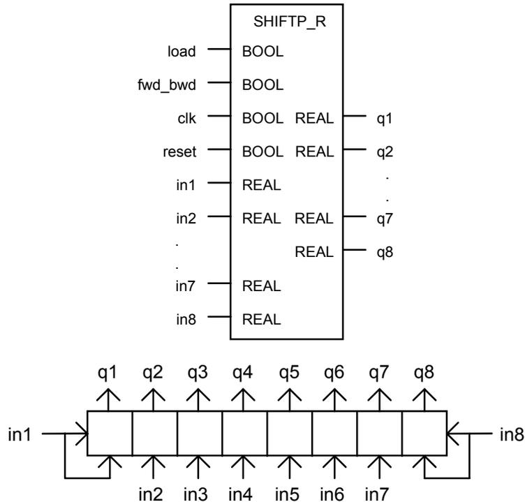
**Short description:** Bidirectional real shift register with 8 parallel inputs and outputs
