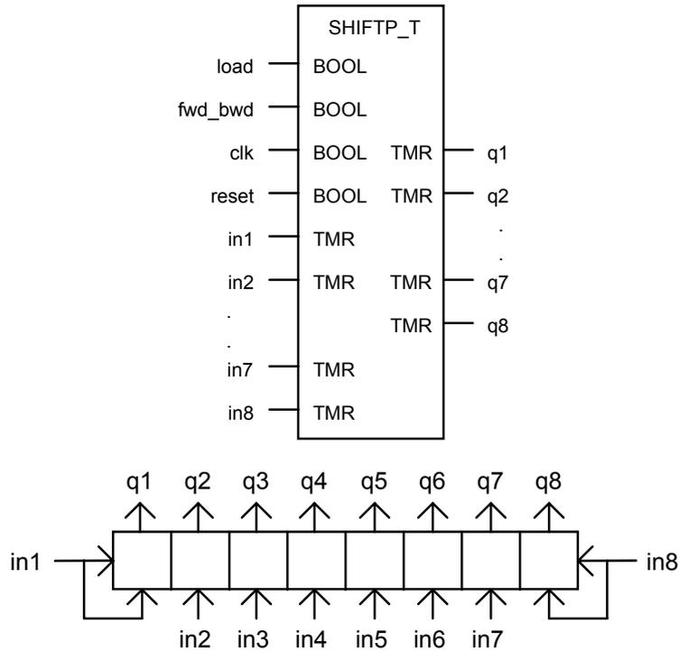
**Short description:** Bidirectional timer shift register with 8 parallel inputs and outputs
