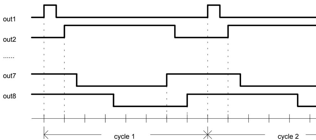
Short description: Multiple digital oscillator with variable duty-cycle
