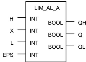
Short description: Alarm detection for an analog (integer) variable
