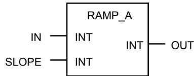
Short description: Ramp limiter for analog signals
