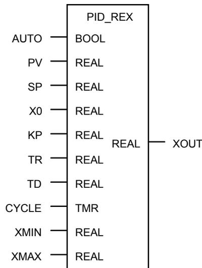
Short description: PID controller with real I/O, EXOR version
