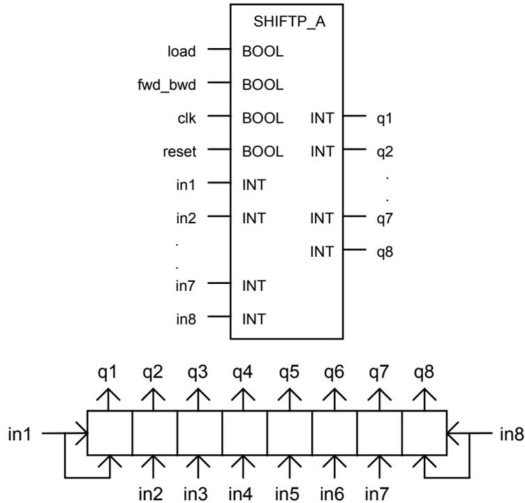
**Short description:** Bidirectional analog (integer) shift register with 8 parallel inputs and outputs
