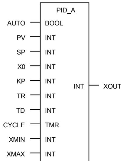
Short description: PID Controller with analog (integer) inputs and output
