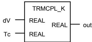
Short description: Thermocouple linearization/compensation for K type
