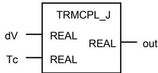
Short description: Thermocouple linearization/compensation for J type
