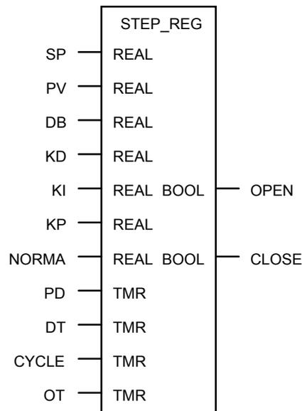
Short description: 3-state controller with PID velocity algorithm
