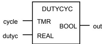
Short description: Digital oscillator with variable duty-cycle
