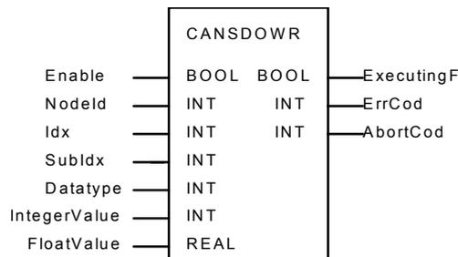
**Short description:** Write one variable in CANopen node using SDO protocol
