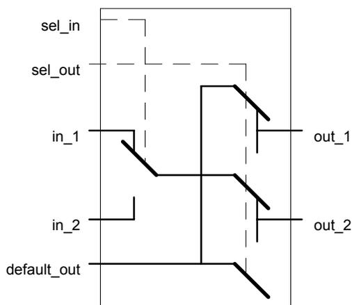
Short description: Double independently operated analog switch with two inputs
