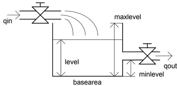
Short description: Reservoir (integrator) with input and output flow
